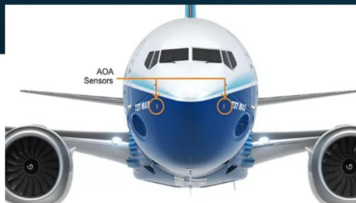
Boeing 737 MAX planes are quipped with two angle of attack (AOA) sensors on either side of the fuselage nose, but a flight control software fix called MCAS was relying on data from just one of the sensors in the Lion Air crash in 2018, authorities said. (Boeing)
