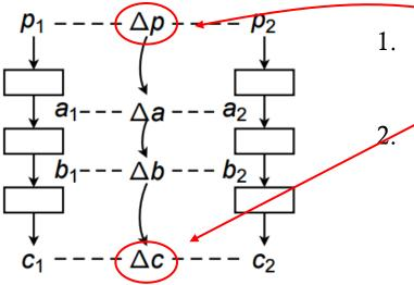
Observe the difference between two ciphertexts as a function of the difference between the plaintexts Find the highest probability differential input (characteristic) which can be traced through several rounds
