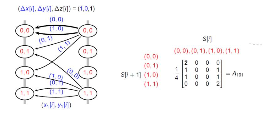
Probability:  $\operatorname{xdp}^+(\Delta x, \Delta y \to \Delta z) = LA_{w[n-1]} \cdots A_{w[1]}A_{w[0]}C$   $w[i] = \Delta x[i] \parallel \Delta y[i] \parallel \Delta z[i], \ 0 \le i < n,$   $L = [ \ 1 \ 1 \ \cdots \ 1 \ ],$  $C = [ \ 1 \ 0 \ \cdots \ 0 \ ]^T.$  (credit to N. Mouha)
