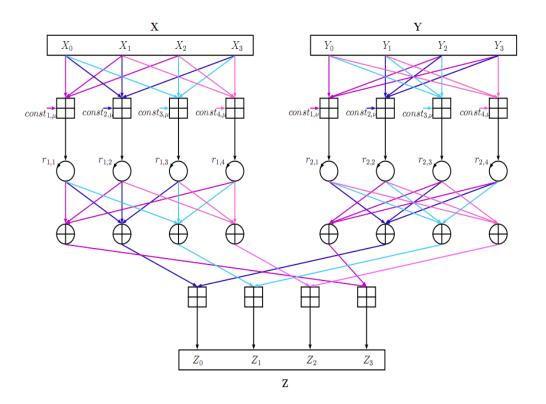
X, Y and Z - 4-tuples of  $\omega$ -bit words ( $\omega = 16, 32, 64$ )
