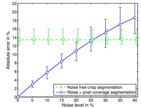
**Left:** (top) Synthetic test objects. (middle) Part of object with 30% noise added. (bottom) Coverage segmentation result for 30% noise. **Right:** Average absolute error of coverage values of object *border pixels* for different noise levels. Lines show averages for 50 observations and bars indicate max and min errors.
