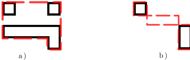
Figure 1: When considering a set of multiple polygons, the rectilinear polygon that contains all of them and is of minimal area: a) may be simple, and therefore the orthogonal hull, b) may not be simple, and is thus not the orthogonal hull.
