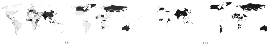
Figure 2: (a) Loaded image with highlighted higher and lower population density converted to Gray color space; (b) applied blur function.
